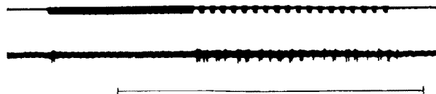
Fig. 1. Responses recorded from the cockroach femur to vibration with a frequency of 1000 c.p.s., partly in pulses of 30/sec.
